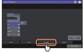
During printing, the button for the drawer from which the paper is fed is highlighted. When you have finished checking, press [Close]. The menu returns to the one shown before you pressed [Job Status].
